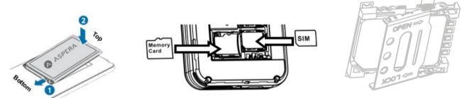
Slide SIM tray cover to the right and lift to open it. Insert SIM then close and slide
